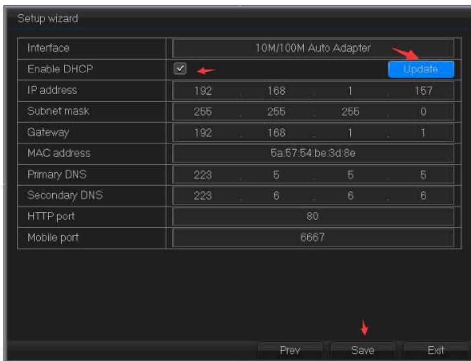
【DHCP Enable】 Obtain IP address automatically.
