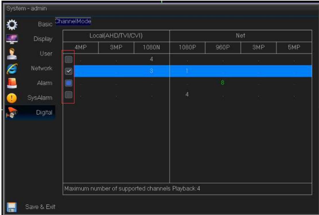
Note: High resolution modes can be compatible with lower resolution cameras; lower resolutions can't be compatible with higher solutions cameras. For examples: analog channel 4\*1080P can connect with 1080P cameras and also 720P cameras.
