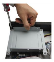
b) Get a compatible SATA HDD. Slide the HDD to the bracket, and fix it with two screws for each side. There are three screw holes per side on the bracket, and you can choose two of them to secure the HDD.
