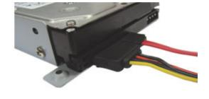
d) Screw the HDD bracket back to the DVR base.
