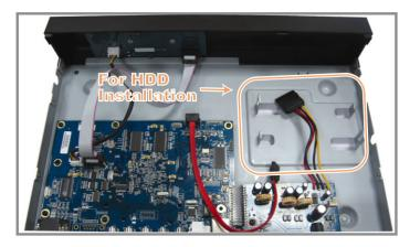
Step 2: Get a compatible HDD, and connect it to the power connector and data bus connector.
